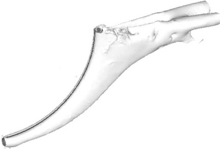
FIGURE 11. Wake topology for the flow past the concave configuration at  $Re = 100$ ,  $\lambda_2 = -0.01$ .
